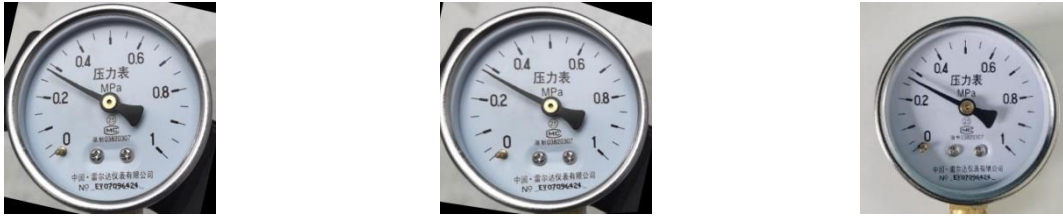
(a) Before perspective transformation image (b) After perspective transformation image (c) Template matching instrument image Figure 4 Instrument tilt correction
