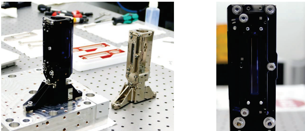
Figure 7. SLITA flight model compared with the SLITA structural model (left). SLITA detail showing the double slit device (right).
