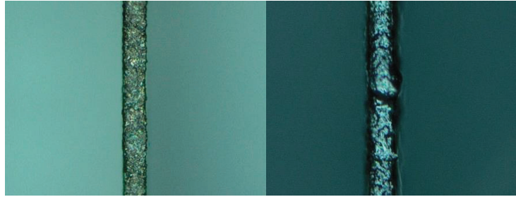
Fig. 7. Cross section of a 38µm aluminum foil coated on both sides, magnification of x100. Left: Acktar Magic Black coating. Right: Black paint.
