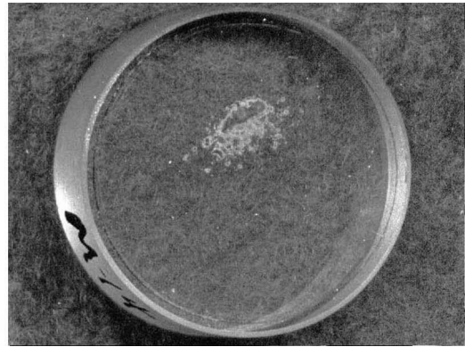
Fig.18. Coating damage on laser turning mirror.
