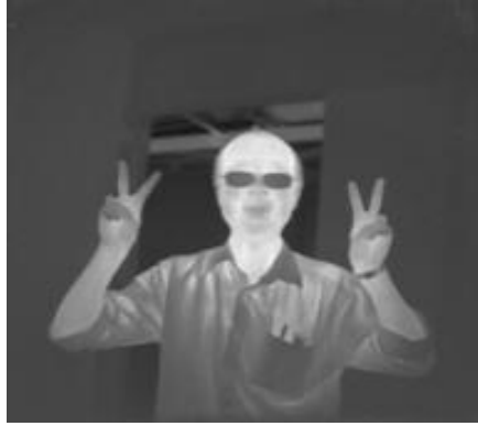
Fig. 7. The measured QE of the C-QWIP FPA (dashed curve) and the spectral shape of an edge coupled detector (red curve) at 3V (left). The QE of the FPA is 26.3% at 5V based on single detector characteristics. The image taken by the FPA at NASA GSFC is on the right.
