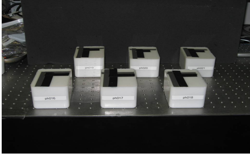
Figure 2: Examples of the standardized phantom constructs made of silicone and nigrosin for the NTROI study.
