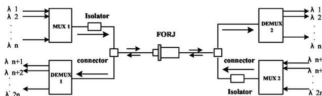
Fig. 1 Principle of dynamic data transmission system.
