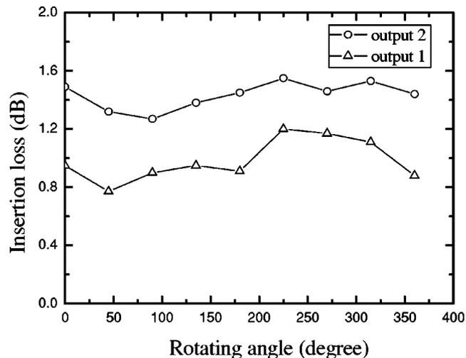
Fig. 4 Relationship between the insertion loss of DDTS and its rotation angle.
