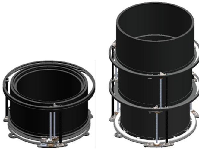
Fig. 7 Concept of the SSTL telescopic deployment barrel. 6
