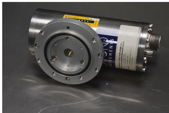
Fig. 4 Photograph of the Iron X-ray tube used as a perpendicular X-ray tube in this work.
