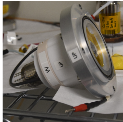
Fig. 5 Photograph of the tungsten X-ray tube used as a parallel X-ray tube in this work.
