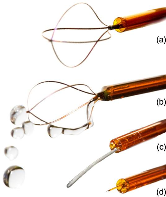
**Fig. 3** Miniature ureteroscope tip with device demonstrations: (a) 1.3-Fr stone basket insertion, (b) stone basket insertion with saline flow through separate channels, (c) guidewire insertion, and (d) 100- $\mu\text{m}$ -core (170- $\mu\text{m}$  OD) delivery fiber insertion through central channel.
