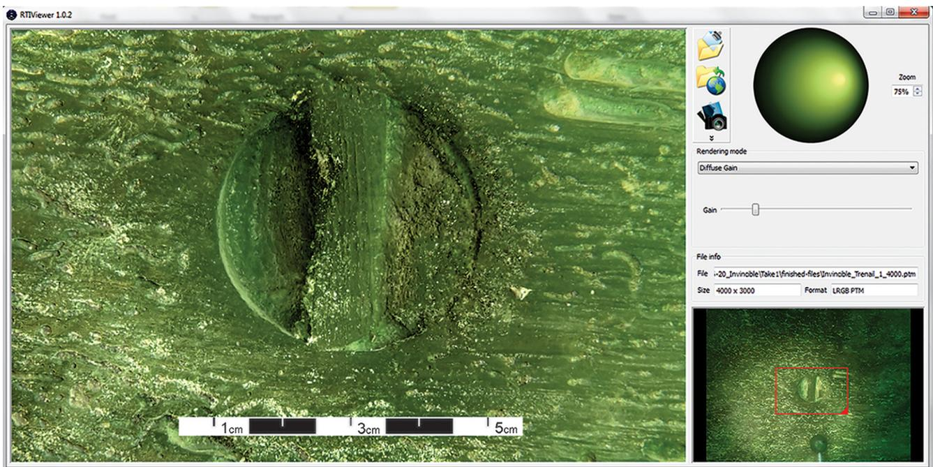
**Fig. 12** Screen-capture from RTIViewer software render of the first polynomial texture map (PTM) produced from UCH using highlight image capture free-form URTI methodology: a treenail from the HMS Invincible.
